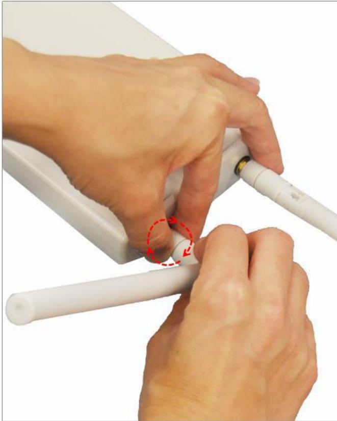
2. Tighten the antenna connectors by turning clockwise. Zcomax recommends fixing one antenna in a horizontal position and the other vertical. This will give 30 dBi of isolation between the radios.
