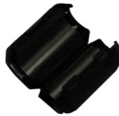
2. Lay the Ethernet cable into the core, usually within 2 to 3 inches of the connector. You may have to experiment with the final location depending on the effectiveness of the high frequency abatement.
