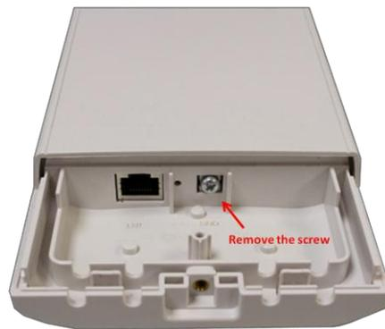
2. Put the grounding wire on the grounding terminal at the bottom of the ZAC 1023. Tighten the screw.
